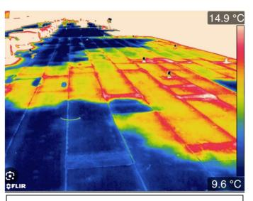
Finding #2: Potential Seam & Fastener Anomalies - Severity: Critical
