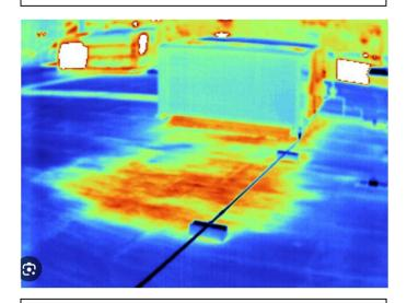
Finding #3: Failed membrane seam - Severity: Medium
