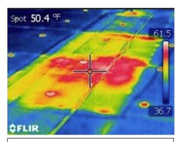
Finding #1: Significant Subsurface Moisture Detected - Severity: Critical
